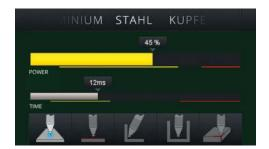
You select the material - steel, aluminium or copper on the modern touch screen and specify the task: surface, edge, fillet, groove or corner and off you go.
